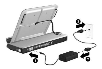
Connecting the Expansion Base to AC Power
